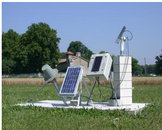
Plate 1: Aeronet sun photometer system (NASA, 2000)
